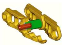
**Track.** The 345C L comes standard with the new grease lubricated track called GLT4. The track links are assembled and sealed with grease to decrease internal bushing wear, reduce travel noise and extend service life lowering operating costs.
